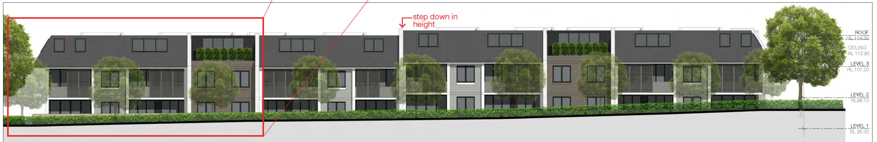
East Elevation, Building B with annotations (Excerpt DA 3.04, Hycorp Design in collaboration with Amglen)
